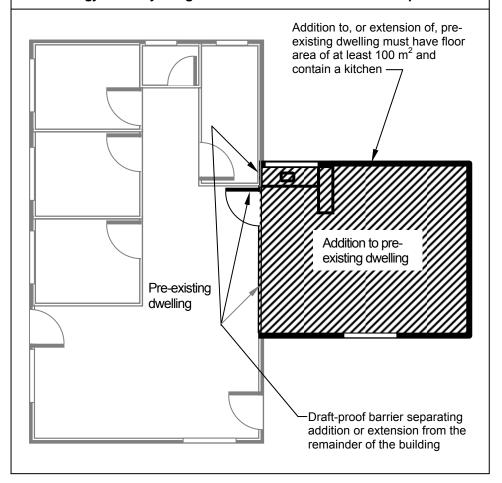
Example 2—compliance with certain requirements of ACT 7.1.2(a)(ii) and (b), incorporating a small amount of floor area of a pre-existing dwelling into the relevant floor area of an addition or extension to the dwelling. This is relevant where house energy efficiency rating software is used to demonstrate compliance.
