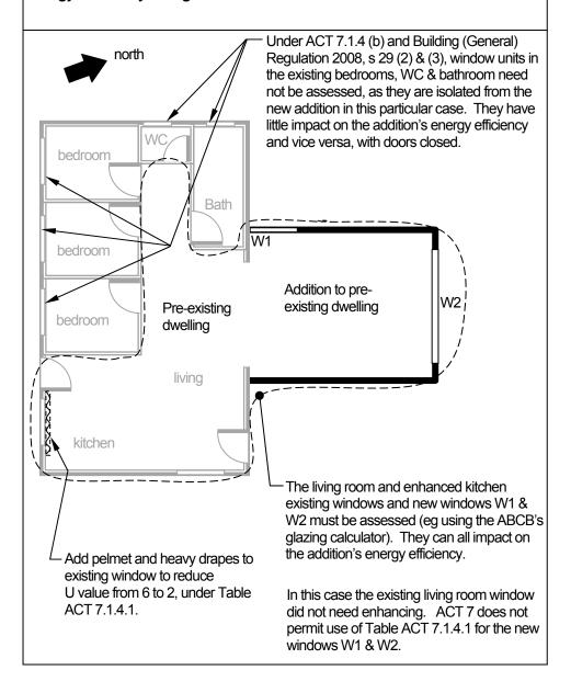
Example 2—plan showing a method of compliance with certain requirements of ACT 7.1.4(c), in assessing window energy efficiency as part of a deemed-to-satisfy alternative to using house energy efficiency rating software, where the ABCB's 2009 glazing calculator may be used rather than the current calculator, as a concession.
