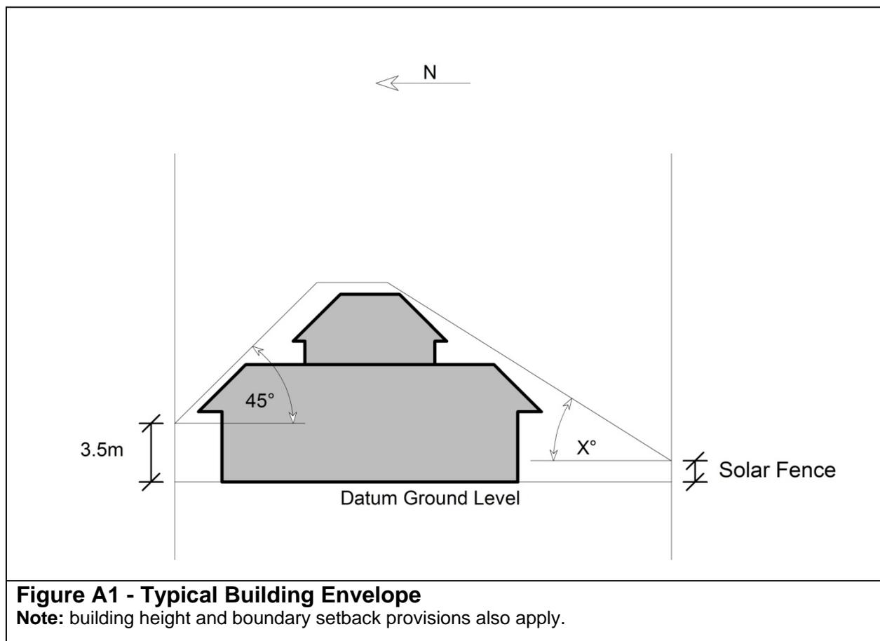
**Figure A1 - Typical Building Envelope**
