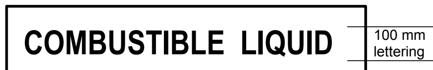
Figure 2.6—Placard for C1 combustible liquids
