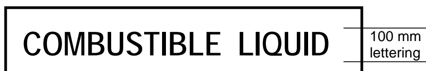
Figure 2.6—Placard for C1 combustible liquids
