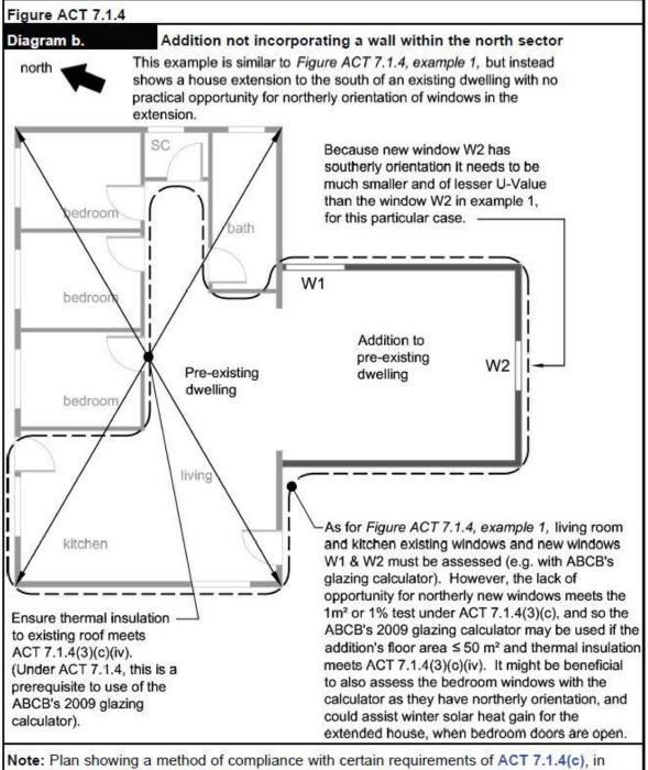
**Note:** Plan showing a method of compliance with certain requirements of ACT 7.1.4(c), in assessing window energy efficiency as part of a deemed-to-satisfy alternative to using house energy efficiency rating software, where the ABCB's 2009 glazing calculator may be used rather than the current calculator, as a concession.
