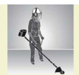
The heaviest part of this brush cutter is located behind the wrists and the weight is supported by a harness.
