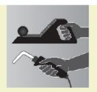
Select tools that can be held with a neutral wrist or in a handshake position with the hand adopting a comfortable (not too open or too closed) grip. Orient jigs and fixtures holding the workpiece so that the wrist does not have to bend.
