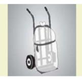
A trolley can eliminate many of the risks involved in manual handling, however, the load will still need to be manoeuvered onto the trolley and through the workplace.
