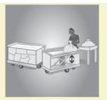
A self-adjusting base in the laundry tubs reduces the need for bending, twisting and reaching during unloading.
