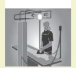
An overhead suspension system reduces the forces required to use the iron.
