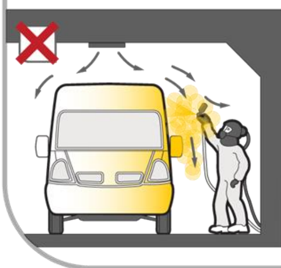
FIGURE 7 The operator is exposed to overspray and reaching above shoulder height can cause discomfort and injury to the body
