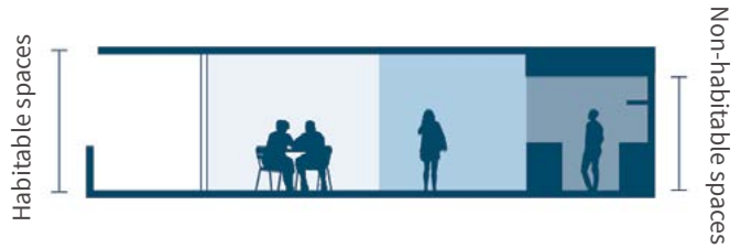
Figure 14: Determine ceiling heights in consideration of the depth and function of the space.
