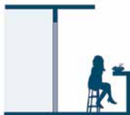
The balustrade can be designed to include usable furniture such as table or seating on narrow balconies.
