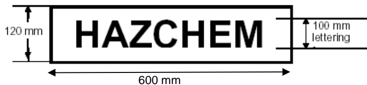
Figure 13.1 Form and dimensions of outer warning placard
