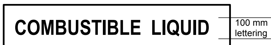
Figure 2.6—Placard for C1 combustible liquids
